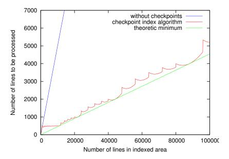
Fig. 4. Expected number of trace file lines to be processed for a jump. The maximum checkpoint count m is 10 and the initial checkpoint distance d is 1000 lines here.
