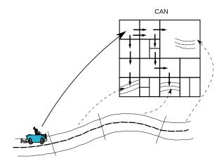
Figure 1: Naive application of CAN to a TIS. Dashed arrows show how the road segments are mapped into the structure. Bold solid arrows indicate the hops in the overlay necessary, for the peer in the left top zone, to fetch the data.
