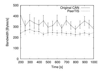
Figure 3: Average peer load with 20 % penetration ratio.
