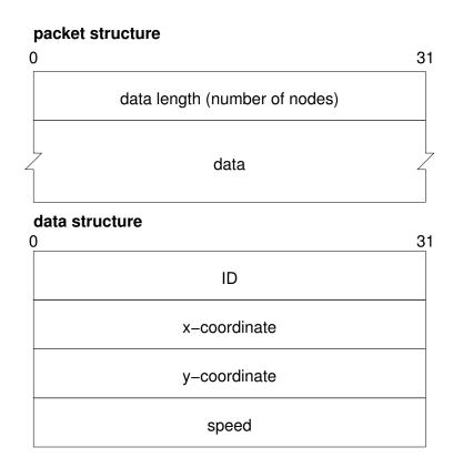
Figure 3.3: Packet structure for movement updates of nodes within the scenario.
