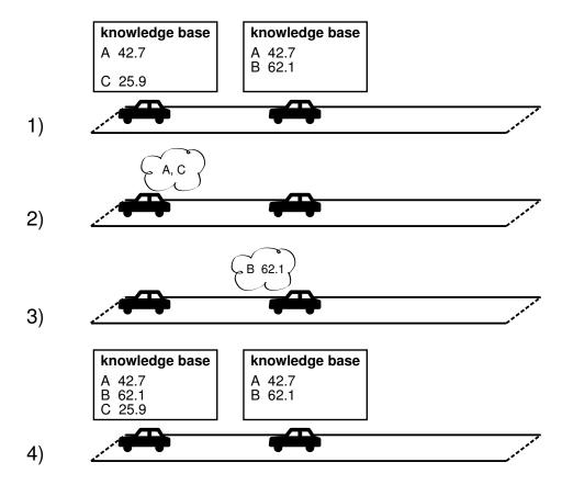
**Figure 2.2:** Implicit information exchange. In 1) two cars with different knowledge bases meet. In 2) the left car propagates its own knowledge. By comparing this announcement the right car can differentiate which entries it owns and are thus needed by the left car. In 3) it transmits the missing entry. Finally, in 4) the left car has updated its knowledge base.
