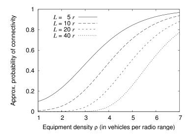
Figure 4.2: Approximated probability of radio connectivity dependent to the equipment density.
