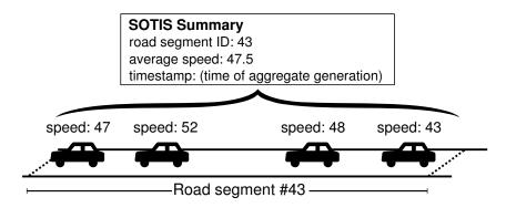
Figure 2.3: Per-segment vehicle velocity summarization in SOTIS.
