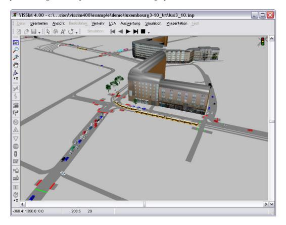
Figure 3.2: Screenshot of the main window of the traffic simulator VISSIM.
