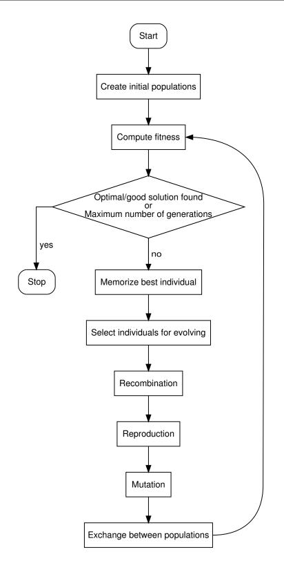
Figure 6.5: The procedure of a GA based optimization approach.
