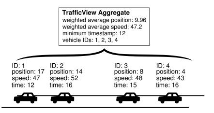
**Figure 2.4:** An aggregate over four vehicles in TrafficView; the calculation of the weighted averages here assumes that the aggregating vehicle is at position 0.
