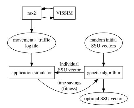
Figure 6.3: Toolchain used for SSU placement optimization.
