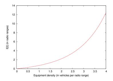
Figure 4.3: Estimated length of chain dependent to the equipment density.
