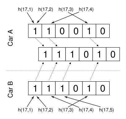
Figure 7.1: Generation and merging of FM sketch aggregates.
