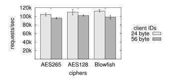
Fig. 4. Measured processing speeds.
