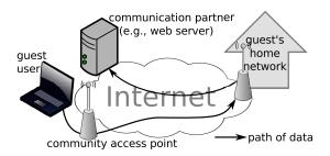
Fig. 1. WiFi sharing approach using triangle routing.
